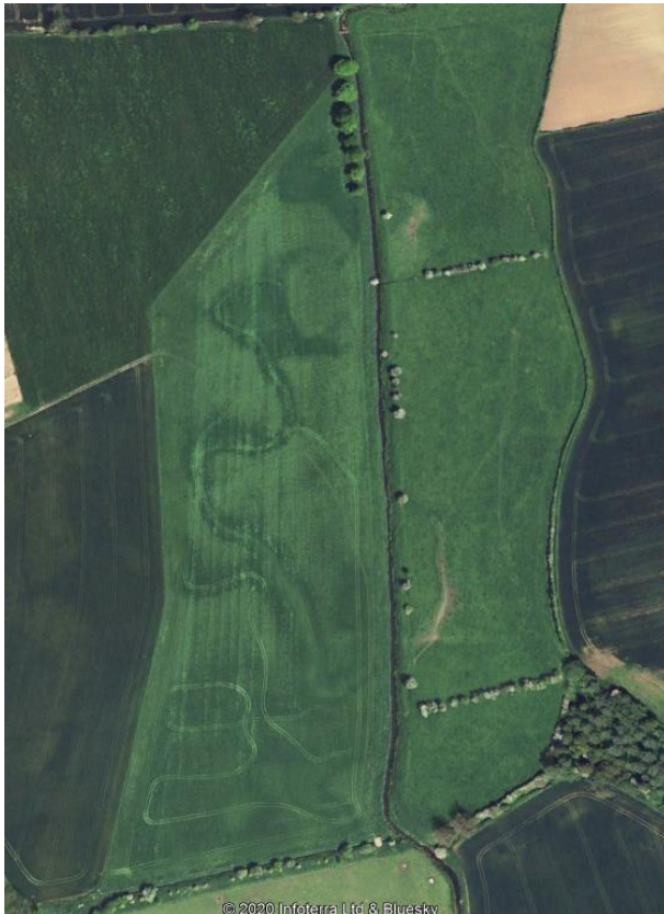
Figure 10: Evidence of former meanders removed by straightening of the River Wiske north of Northallerton [Google Earth Pro]
